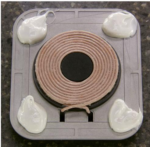
Figure D-2: 100% Silicone applied to transmitter
